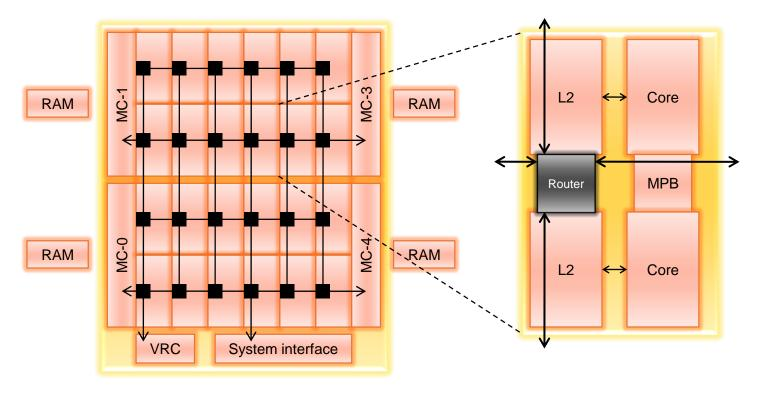
24 \* 2-core tiles On-chip mesh n/w Non-coherent caches Message passing buffer
